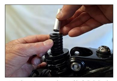
15. To change it, remove the seat, (don't dis-lodge the spring), remove bump-stop, insert small spring (start with lowest #) into the main spring, insert the correct bump-stop and retry. Repeat if nec. noting section 14.
