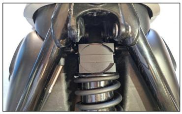
7. Clean top of shock to remove any grime. Peel off adhesive backing, position it onto shock. You will not be able to re-adjust its position once in place, accuracy is recommended! (FOX shock shown).
