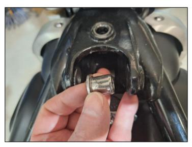
Remove the chrome bush from the RH seat mount hole and apply a smear of grease to the outside circumference and re-insert.
