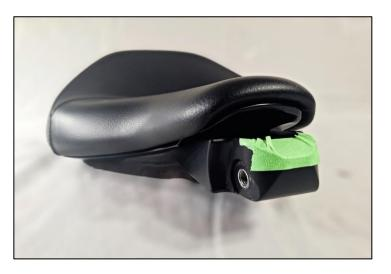
5. Fit the new seat bracket to the seat and adjust to your preferred riding position. Place tape on the nosing as shown for protection during installation.
