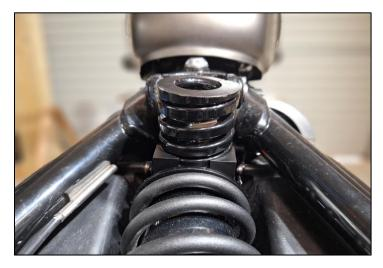
10. Place the main (large) spring into the circular cutout in the top of the spring base mount.
