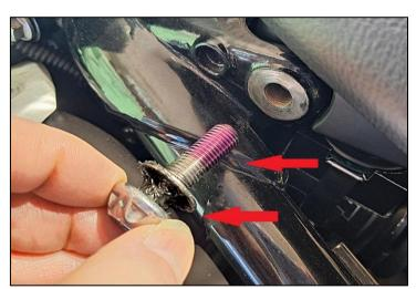
16. When finished fit the 2 front bolts. Right bolt insert and tighten (no grease or thread-lock). Left bolt plus supplied washer, apply grease to top part of shaft and both sides of washer, apply thread-lock to thread, insert and tighten till firm (still allowing seat rotation).
