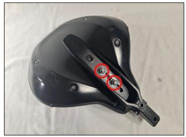
4. Remove the 2 nuts and washers securing the seat bracket to the seat.
