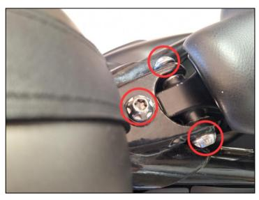
1. Remove these 3 bolts to release the seat and seat bracket. Requires a Torx 50 bit. The rear of the tank will need to be raised on 12 litre tank models.
