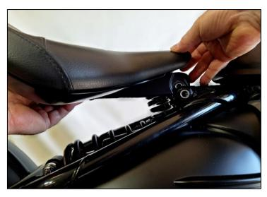
12. Keeping the rear of the seat low, place the seat assembly over the spring, then raise the seat rear and line up the bracket hole with the bike chassis holes.
