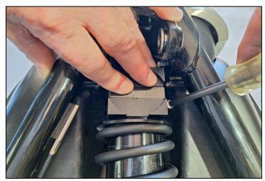
9. Once thread is just started rotate the clamp so the screw is to the side, ensure strap fits into the recess on top of the spring base mount and tighten firmly.
