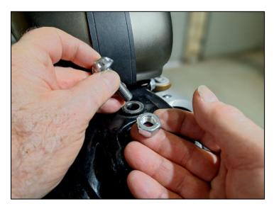
3. Using supplied locknut, re-instal seat bracket top bolt, it has no further use other than cosmetic.
