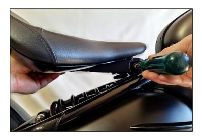
13. Insert a suitably sized screwdriver through this hole to hold the seat assembly in place temporarily. It's quicker and less fiddly.
