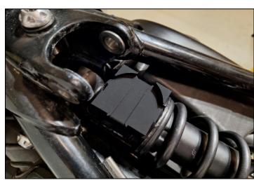
6. The spring base mount sits on the shock upper casing, against the centre flange and level with the bike. Do a dry test run first. (OEM shock shown).
