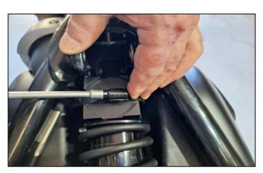
8. Open up the clamp and wrap it around the shock and base mount. It's easier to thread the strap into the worm screw if you do it on top of the mount.
