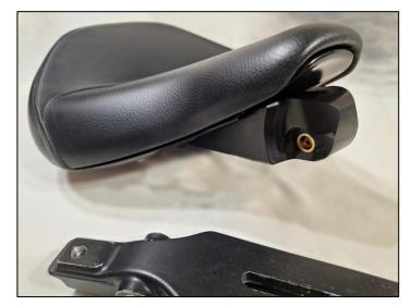
4. Swap the old seat bracket for the new seat bracket and adjust to your preferred riding position. The pivot pin bearing is oil-impregnated bronze in composition and does not require additional lubrication.
