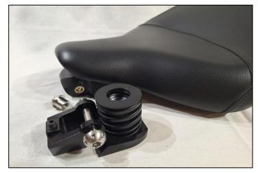
8. Put the spring bottom mount, main spring with a bump-stop inserted (see section 9) and seat bracket into one assembly and secure with the pivot pin.
