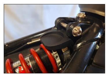
5. Place spring bottom mount into position on the bike and slide pivot pin through from LHS, fit nut to RHS to hold it in place.
