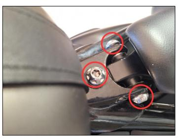
1. Remove these 3 bolts to release the seat and seat bracket. Requires a Torx bit. The tank will need to be raised on 12 litre models.
