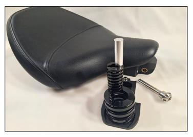
13. To change the spring rate, re-fit the strap, remove seat assembly, remove large bump-stop, insert small spring into the main spring (#1 is softest) insert small bump-stop and retry. Repeat as nec. noting section 12.
