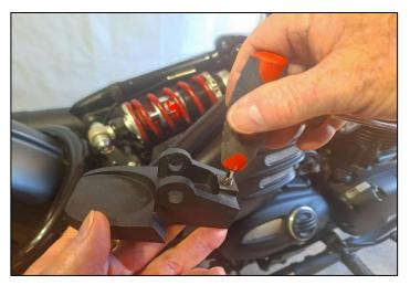
7. If gap is too small, remove spring bottom mount and turn set screw out, re-checking until that minimum clearance is achieved. Also see section 14.
