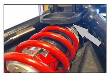
6. Look underneath the mount to see if there is contact between it and any part of the shock (torchlight will be handy). Keep a minimum gap of approx. 1/8in or 3mm between the two. (If gap is larger, leave it at that gap).
