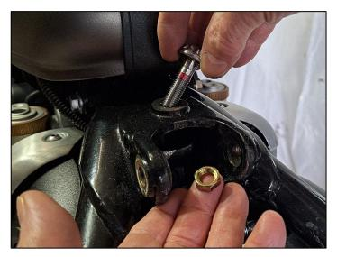
3. 9 Litre tank models only - Insert thin ½ nut to the underside of front seat hole, (be careful not to drop it down the centre of your bike) fit original screw with thread-lock to the top few threads only and tighten. For 12 Litre tank models, no screw/nut required, just refit the black cover plug.
