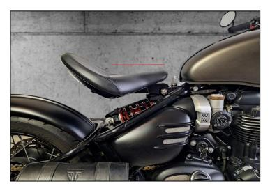
14. If the angle of the seat isn't correct when seated, you can change the angle with the set screw provided you adhere to minimum clearance as per section 7. As a guide the seat should be slightly nose-up.
